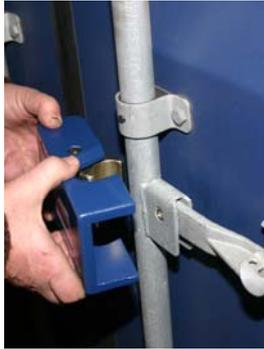
The CC FixLock 3 being fitted above the handle and pressed against the container door.
