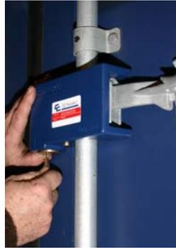
Locking: Push the lock up and turn the key. Make sure the lock is *engaged*.
